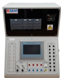
EA10: Platine Automate Siemens S7-1200
